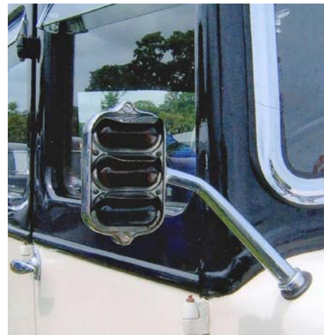
Wilcot traffic light direction indicators
